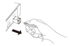
2. Pull down the latch and remove the module.
