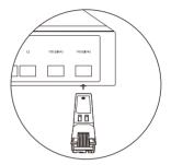
$2. \ \ \text{Gently push the module into the slot until you hear a click. Then, insert the RJ45 \ network \ cable.}$
